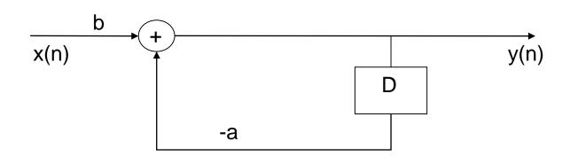
Three basic elements in block diagram: adder(加法器), multiplier/amplifier(常系数乘法器), unit delayer(单位延时器)
