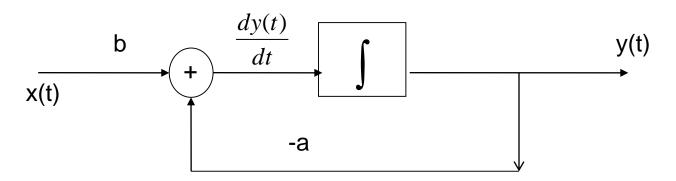
Three basic elements in block diagram: adder(加法器), multiplier/amplifier(常系数乘法器), integrator(积分器)
